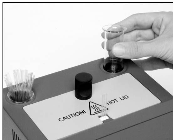
Figure 3. Mounting the glass Capillary Holders.
