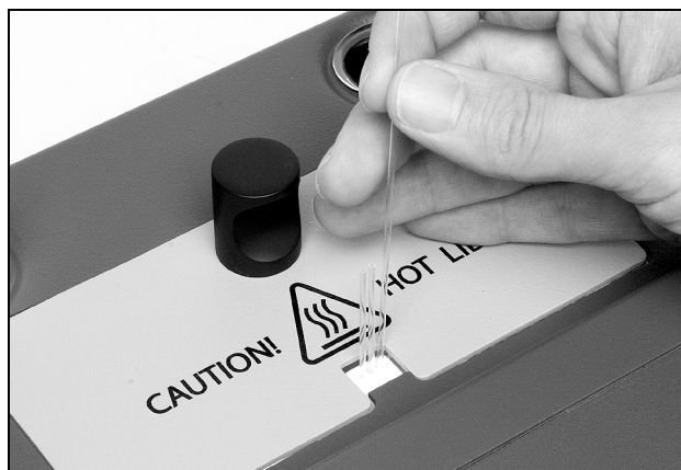
Figure 9. Loading capillaries into EZ-Melt.
